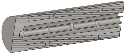
Figure 4: Structure with four accelerating gaps.
