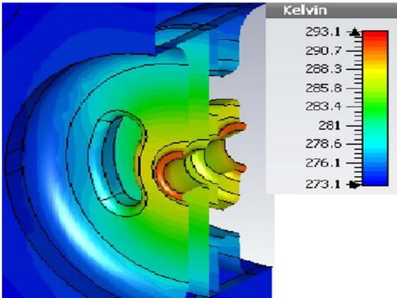
Figure 7: The view of the BAS section and temperature distribution ,water flux equal 0.3 l/s.
