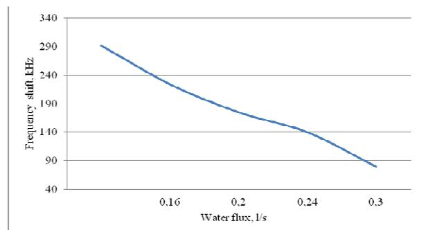
Figure 5: Frequency shift versus of water flux.
