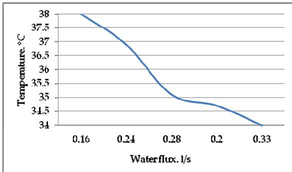
Figure 6: Maximal temperature versus of water flux.
