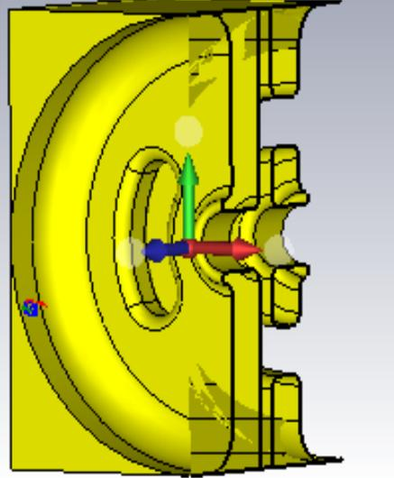
Figure 2: The geometry of the BAS cell, the shell material – copper.
