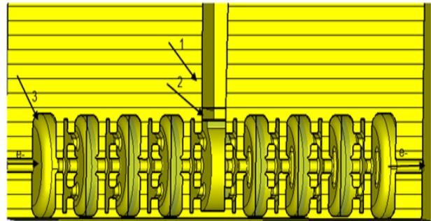
Figure 1: General view of the accelerating structure, 1 – coupler, 2 – power feeding waveguide, 3 – regular accelerating cell.
