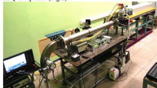
Figure 1: Nd-YAG laser at the test bench.
