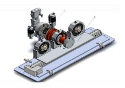
Figure 2: System for remote replacement of liquid and gaseous targets (three in total).
