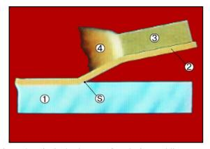
Figure 3: Principal schemes of explosion welding process with an angle between metal sheets 1 - base plate; 2 – cladding plate; 3 - explosive; 4 - detonation products; S point (line) of contact of surfaces during welding.
