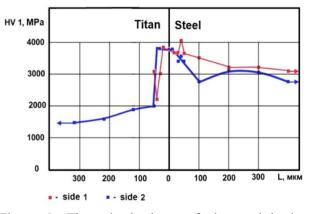
Figure 5: The microhardness of the steel-titanium boundary after explosion welding.
