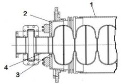
Figure 1: Scheme of combined adapter connection with a cryogenic module: 1 – steel shell; 2 - electron beam welding or argon arc welding connection of shell with steel flange of adapter; 3 - steel flange; 4 - niobium tube.
