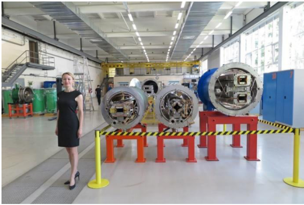
Figure 5: Series dipole magnet (left) and doublet (center) for NICA booster, and pre series dipole magnet for NICA collider (right).
