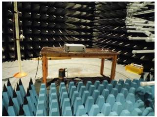
Figure 5: Test set-up for radiated susceptibility.
