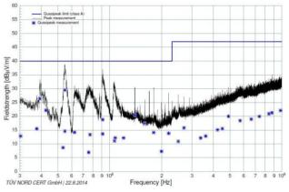
Figure 1: Radiated emission. Vertical antenna polarization.
