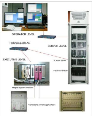
Figure 1: KSRS magnet system control.
