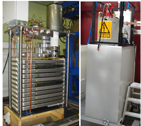
Figure 5: Direct switch solid-state 110 kV modulator: - out of oil-tank with test resistive load on the left and - in the oil-tank with the klystron on the right.
