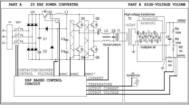
Figure 1: The high-voltage source block-diagram.
