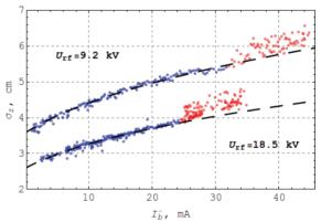
Figure 4: Bunch length as a function of beam current at energy E=480 MeV.
