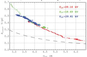
Figure 6: Longitudinal loss factor at energy E=480 MeV.
