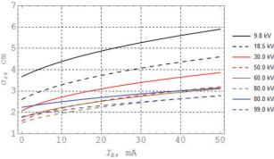
Figure 7: Bunch length as a function of beam current at different energies and RF voltages.
