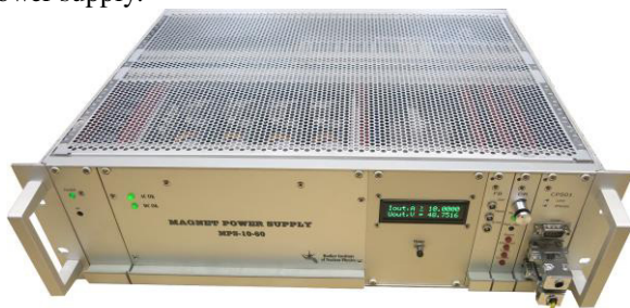
Figure 1: The power supply for corrector magnets.
