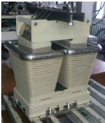
Figure 6: Pulse transformer of the TDS BC1.
