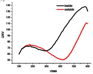
Figure 9: Mean acceleration voltage along radius.
