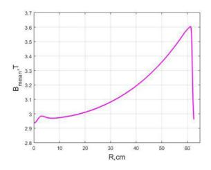
Figure 5: Average magnetic field along the radius.
