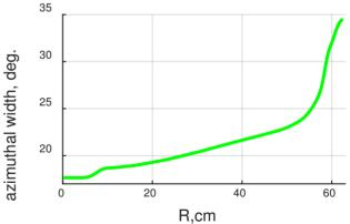
Figure 4: Azimuthal width of sector.
