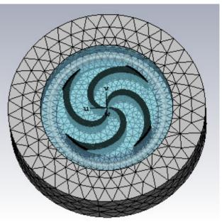
Figure 3: Model of the magnet.
