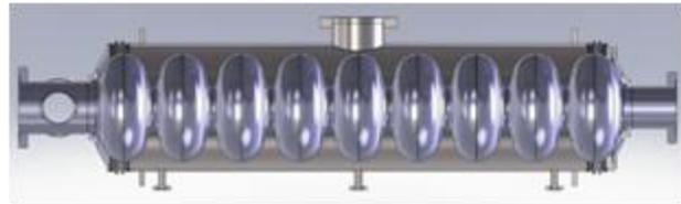
Figure 5: The e-Linac nine cell cavity with jacket.
