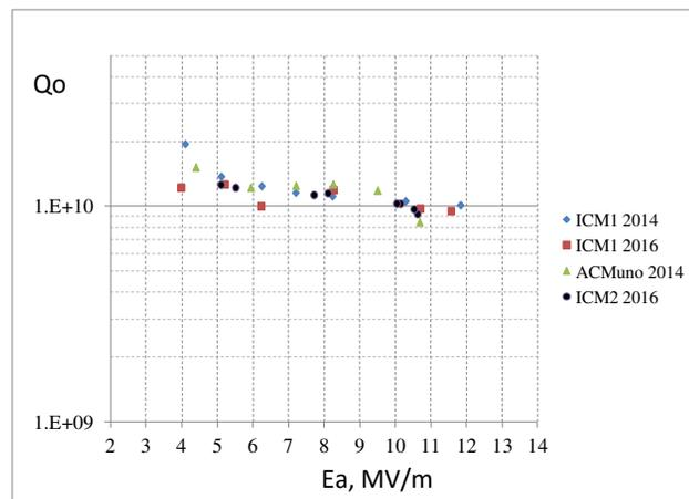
Figure 6: Q-curves of the cavities in eLinac cryomodules.
