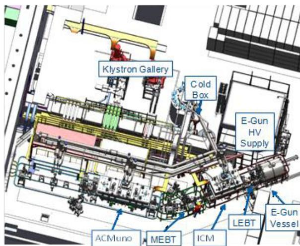
Figure 4: The Phase-I configuration of the eLinac.
