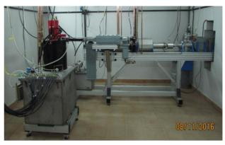
Figure 3: Photo of installed linac at ACCENTR Ltd. Company site, the beam scanner is clearly seen in the right side of the photo.
