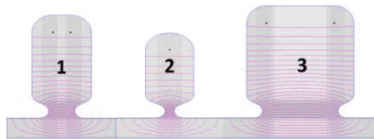
Figure 4: Electric field lines in the optimized buncher.
