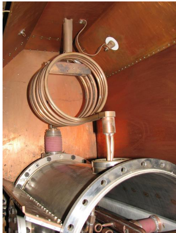
Figure 2: The opened resonator with the replaceable helical part that is connected to the accelerating channel via a feedthrough.
