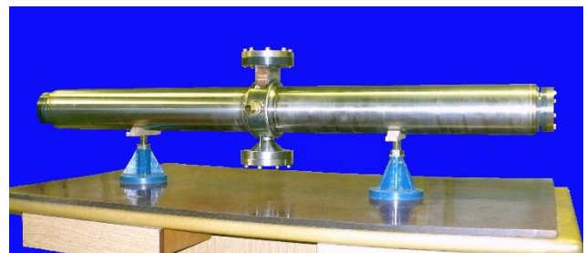
Figure 6: Accelerating structure with cooling jacket.
