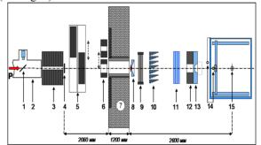
Figure 1: Formation system of INR medical proton beam. 1 – luminophor with TV-camera, 2 - beam channel; 3 - graphite collimator, 4 - the primary scatterer (S1), 5 – beam stop, 6 – beam aperture collimators of 40 and 70 mm, 7 - shielding, 8 – secondary scatterer (S2), 9 - ion chamber, 10 - ridge filter, 11 - energy degrader, 12 – individual collimator, 13 – bolus, 14 - ion chambers in a water phantom, 15 – target isocenter.
