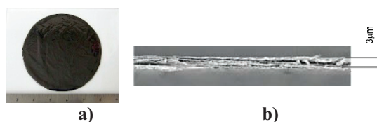
Figure 1: General view of graphene foils: a) fabricated foil; b) graphene cross section.
