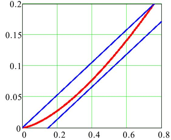
Figure 2: A plot illustrating beam reflection. Strait lines are target borders, the curve is beam envelope.  $\Theta_s^2 = 0.55 \text{ cm}^{-1}, h = 0.15 \text{ cm}, k = 3.8 (t = h/\sqrt{1+k^2} \approx 0.04) \text{ cm}$ , target material is aluminium.
