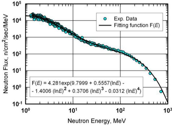
Figure 3: Neutron spectrum from the “bare” lead target measured at the 36.5 m flight path station of the beam #5. The data are normalized to an average neutron production rate of  $2.5 \cdot 10^{14}$  n/s.
