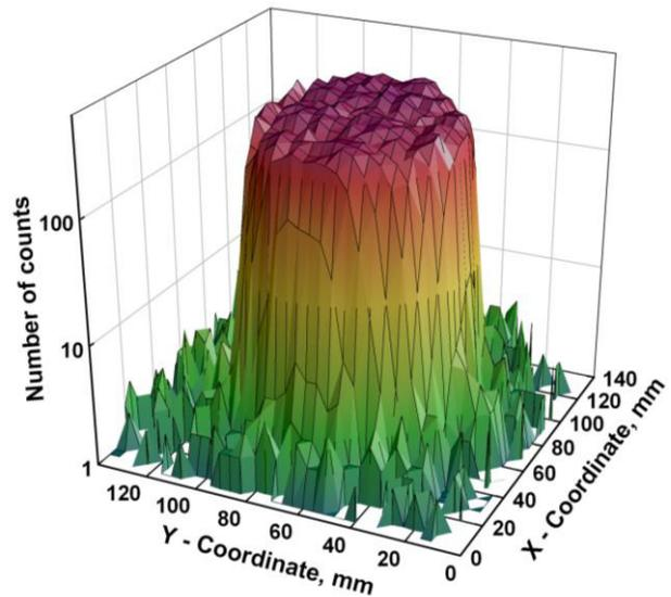
Figure 6: Neutron beam profile measured using MWPC.
