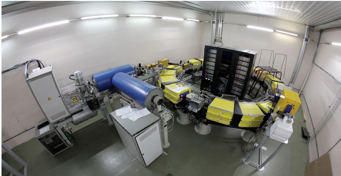
Figure 1: The synchrotron and injection channel for the proton therapy complex “Prometheus”.
