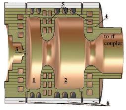
Figure 2: Simplified model of the gun cavity. 1 - half cathode cell, 2 - full cell, 3 - position of photo cathode, 4- cavity copper body, 5 - cooling channels, 6 - stainless steel jacket.
