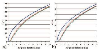
Figure 3: Time dependence of maximal temperature rise of the surface  $T_{smax}$  (a) and relative increase of RF losses (b) for rectangular (blue traces) and accretive with  $\tau_{c1}$  (red traces) or  $\tau_{c2}$  (green traces)  $P_l$  pulse.
