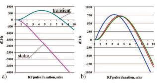
Figure 5: Cavity detuning during accretive  $(\tau_{c1})$   $P_l$  pulse for static and transient approximations (a) and transient detuning for rectangular (blue curve), accretive with  $\tau_{c1}$  (red curve) or  $\tau_{c2}$  (green curve)  $P_l$  pulses (b).
