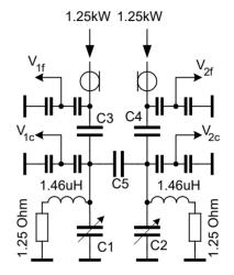
Figure 3: Equivalent schematic of RF cavity/ C1, C2 -82pF, C3, C4 – 22pF, C5 – 8 pF.
