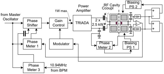
Figure 4: Block-Diagram of RF System 10.94 MHz.
