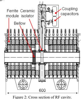
Then these modules were glued in two packages of 8 pieces for each half of the cavity.
