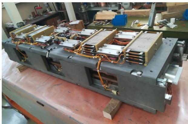
Figure 1: Superconducting 7 Tesla wiggler for DELTA SR Source.
