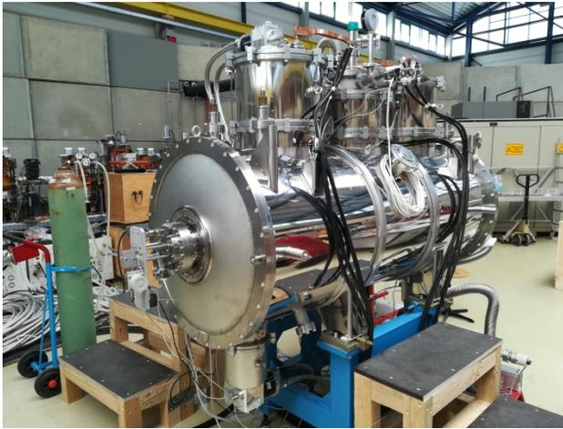
Figure 2: Superconducting 7 Tesla wiggler during site acceptance test in DELTA SR Source.
