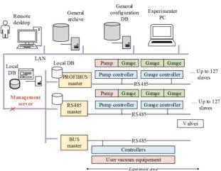
Figure 2: SSRS-4 Control System architecture.
