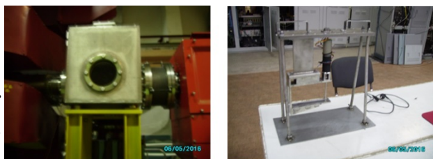
Figure 1: Vacuum box and rotation mechanism of horizontal wire scanner.
