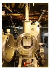
Figure 2: Photo of the multichannel profile detector on the beam-line.
