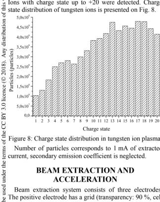
Figure 8: Charge state distribution in tungsten ion plasma. Number of particles corresponds to 1 mA of extracted current, secondary emission coefficient is neglected.
