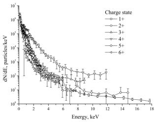
Figure 3: Energy distribution of carbon ions. Target was shifted after each laser pulse.
