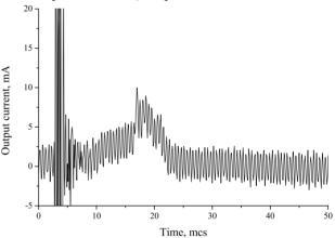
Figure 10: Total ion current at output of the RFQ.
