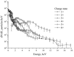
Figure 5: Energy distribution of carbon ions. Target was fixed.
