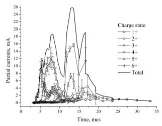
Figure 4: Partial currents of carbon ions. Target was fixed.
