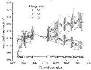
Figure 6: Dependence of ion signal amplitude on time of operation with fixed target.
