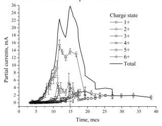
Figure 2: Partial currents of carbon ions. Target was shifted after each laser pulse.
