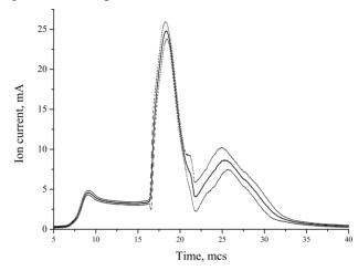
Figure 9: Total ion current at input of the RFO.
