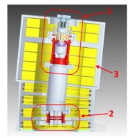
Figure 6: Electron gun for the NICA cooler. 1 – electron gun, 2 – electrostatic lens, 3 - gun solenoid.
