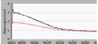
Figure 1: The proton beam cooling at COSY (Julich). The cooling time is about 100 s.
