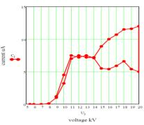
Figure 3: The corona current versus voltage.
