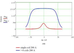
Figure 5: Results of measuring magnet field along cooling section by the hall probe.
