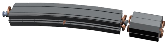
Figure 6: 3D models of a dipole and a quadrupole of the Booster-Nuclotron beam transport channel.
