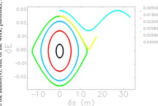
Figure 4: Phase trajectories for synchrotron oscillations.
