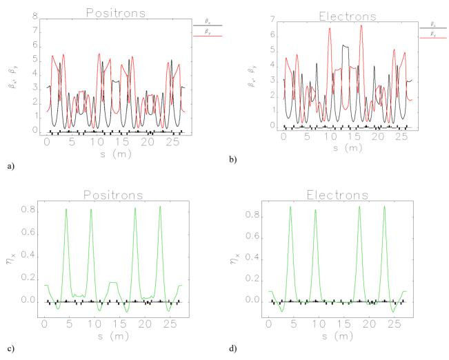
Figure 3: Optical and dispersion functions for Damping ring operation modes: a) positron beta-functions, b) electron beta-functions, c) dispersion of positrons, d) dispersion of electrons.
