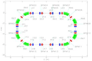
Figure 2: Damping Ring layout.
