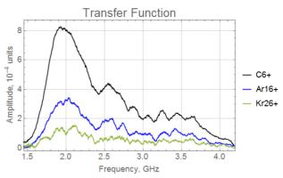
Figure 1: Plot of BTF amplitude. The intensity of carbon beam is  $3 \cdot 10^8$  elem. charges, argon  $-1.5 \cdot 10^7$ , krypton –  $2 \cdot 10^{6}$ .
