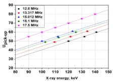
Figure 8: The dependence of voltages measured by the pick-up electrodes on the maximum energy of the X-ray spectrum for different frequencies.
