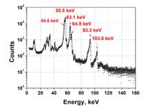
Figure 4: X-ray spectrum from radioactive isotope of <sup>180</sup>Ta.
