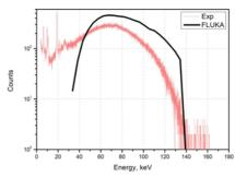
Figure 6: The comparison of the Fluka spectrum (E<sub>electrons</sub> = 140 keV) with the measured spectrum.
