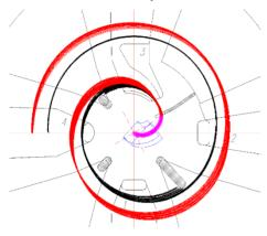
Figure 10: The motion of the injected 15N5+ ion beam on the first turn at the voltage on dees 85 kV (black) and 120 kV (red).
