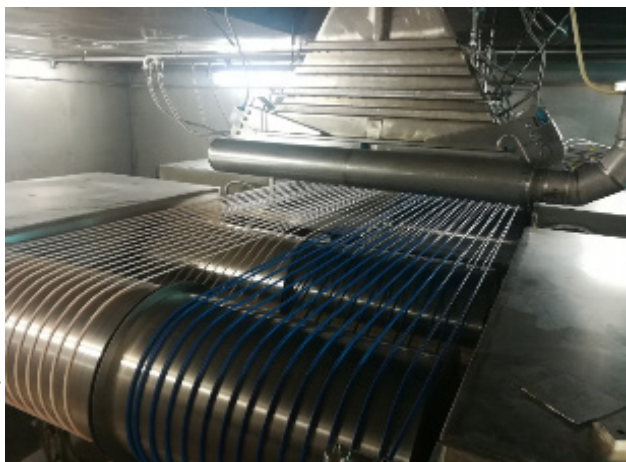
Figure 4: dual line for treatment of wires up to 25 mm 2 by one ELV accelerator.
