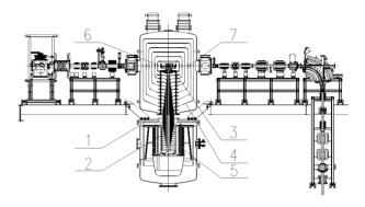
Figure 1: Tandem accelerator circuit: (1) high-voltage source; (2) sectional high-voltage feeder; (3) gas charge – exchange; (4) target electrode of the tandem; (5) rectifier sections; (6) beam H(-); (7) beam H(+).
