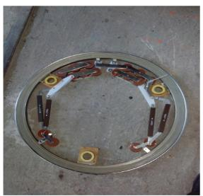
Figure 3: Photo of the rectifier section
