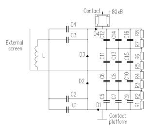
Figure 4: Scheme of rectifier section: (L) coil N = 2000turns; (D1, ..., D4) diodes of the mark SDL-0,55-130 04; (C1, ..., C16) capacitors of the brand FHV-6AN, 3500 pF; (R1, ..., R8) resistors of the brand C3 - 14M.
