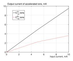
Figure 1: Dependence of the current of accelerated ions on the input impulse current
