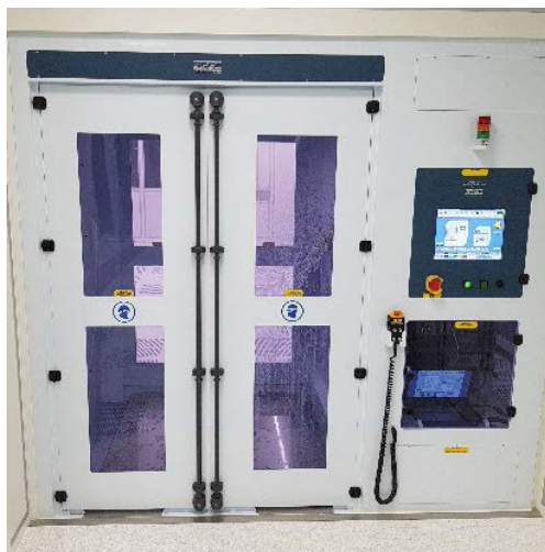
Figure 7: High pressure rinse cabinet: view from ISO-6 access side for loading.
