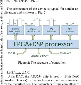
Figure 2: The structure of controller.
