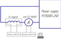
Figure 5: The scheme of dynamic heat releases measurement.
