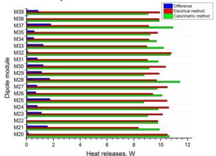
Figure 8: Power of heat releases for the dipole magnets.
