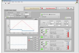
Figure 6: The program for automation of dynamic heat releases measurement: 1 - Controlling buttons, Measurement status bar, 3 - Status of energy evacuation switch, 4 - Data graph, 5 - Cycle parameters, 6 - Heat releases power graph, 7 - Status of first power supply, 8 -Status of second power supply.
