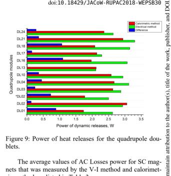
Figure 9: Power of heat releases for the quadrupole doublets.
