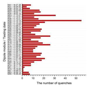
Figure 3: Quenches quantity of the dipole magnets.
