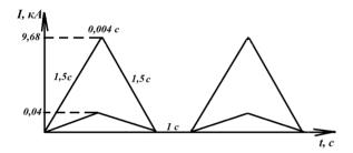
Figure 7: Quadrupole magnet's current cycle.
