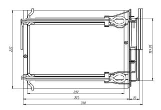
Figure 2: Main view of the multipole magnet.
