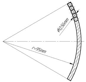
Figure 3: Coil cross-section.
