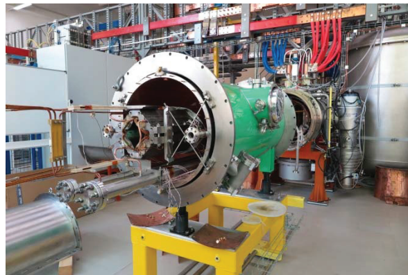
Figure 4: The doublet of the quadrupoles in the cryostat is in preparation for cryogenic measurements.
