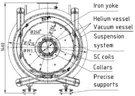
Figure 1: Cross section of the quadrupole.
