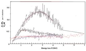
Figure 5: Measured distributions of energy losses of 7 GeV electrons in the multistrip device: the curves 1, 2 and 3 are for the cases of non-oriented, planar orientation and axial orientation, correspondingly. The red points are calculation for non-oriented case.
