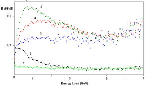
Figure 2: The calculated energy losses:1) in one 2.5 mm long nonoriented strip; 2) in one strip oriented in planar orientation; 3) in nonoriented multistrip, 4) in single crystal with the thickness 15 mm:; 5) multistrip with 6 strips in planar orientation.
