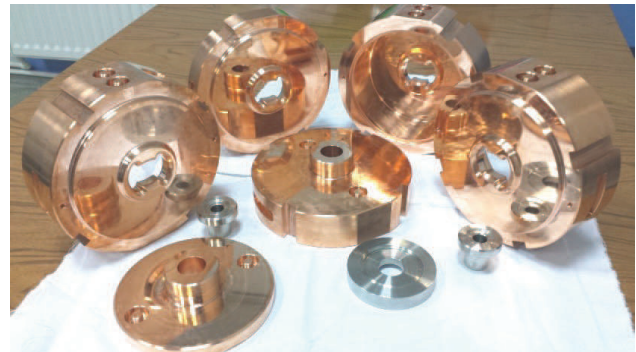
Figure 4: Parts of the cavity after machining.
