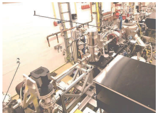
Figure 5: The REGAE beam line. 1 - the cavity, 2 - to the screen.
