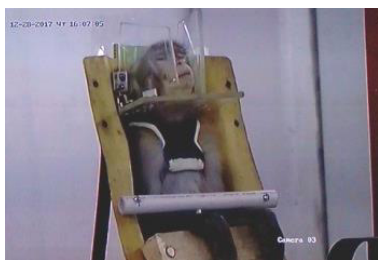
Figure 15: Test animal (a monkey) facing the carbon beam. Through passage of beam across the head with 1 Gydose deposited.
