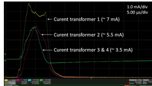
Figure 4: Current transformer signals of He^+ beam, 7 mA-RFQ output, 5.5 mA-IH2 output, 3.5 mA –behind QT4 triplet.
