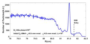
Figure 4: Particles numbers along radius. The entry of the first electrostatic deflector could be placed at r = 81.9 cm.
