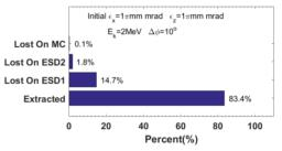
Figure 8: Beam loss distribution in extraction process.
