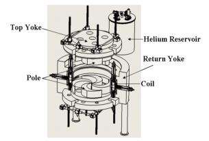
Figure 1: The overall structure of the cyclotron. Table 1: The Main Parameters of the Cyclotron CYCIAE-230
