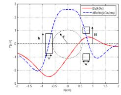
Figure 6: Field distribution in the cross section of the magnetic channel comprised with three iron bars. The size of the bars is given with r=6 mm, w=3 mm, h=8 mm, H=1.25 mm
