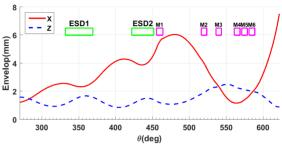
Figure 7: Beam envelop in the extraction process.
