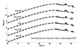
Figure 3: Phase space during the acceleration with different initial RF phase ( $Ø_0$  is the central RF phase), where a first harmonic distribution with maximum B1=2 Gs, center position Rc=79 cm, width  $\sigma$ =8 cm, phase =270°.
