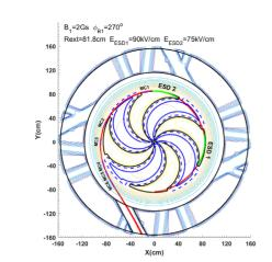
Figure 5: Particle Trajectories in the extraction process passing the electrostatic deflectors (ESD) and magnetic channel (MC) to the outside of the cyclotron.
